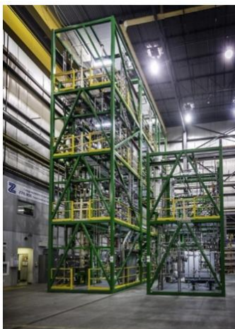
Anellotech's TCat-8 development and testing unit for converting biomass to BTX. Photo courtesy of Zeton Inc.
